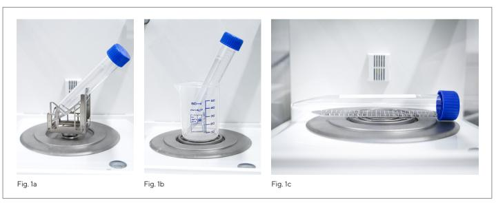
Fig. 1a (Cubis® High Capacity Micro Balance with YSH22 Vial Holder)
